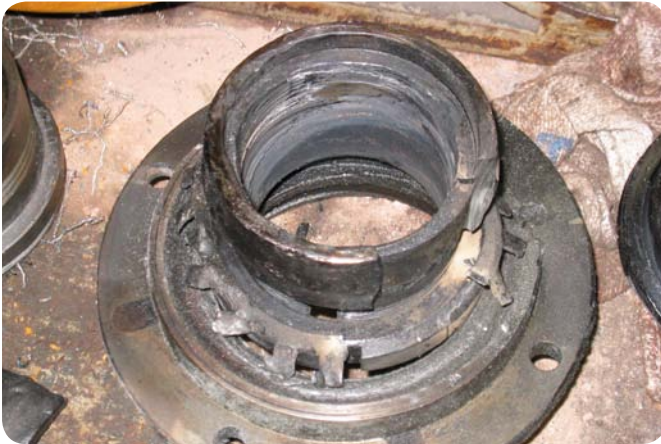
Fig. 12 Advanced wear with rotation of the adapter sleeve on the shaft of a dryer section felt roll bearing. The related high temperature reduced the bearing clearance resulting in uncontrolled preload and, finally, seizure.
