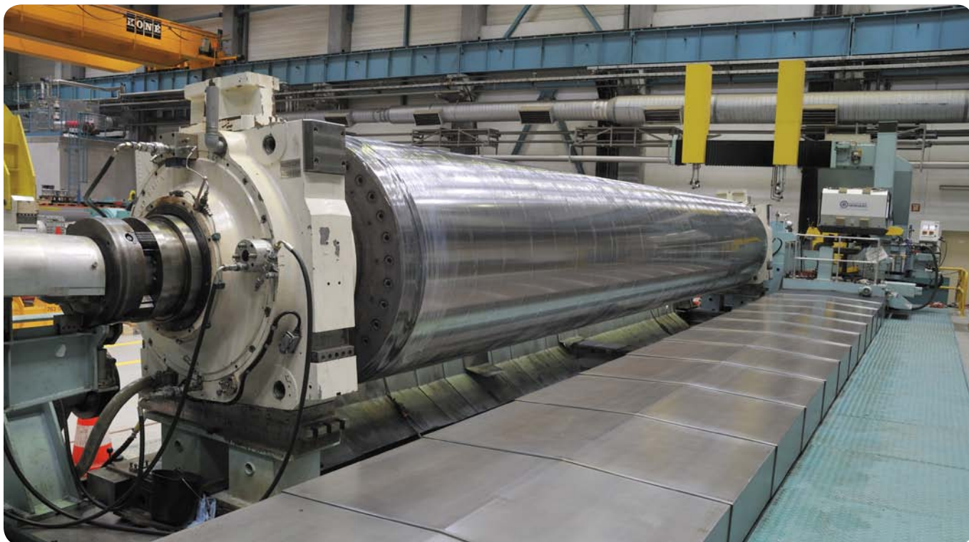
Fig. 7 A roll grinding machine with the roll rotating on its main bearings.
