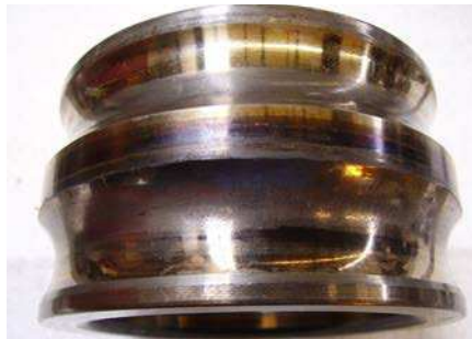
Fig. 2: Path pattern on inner ring raceways
