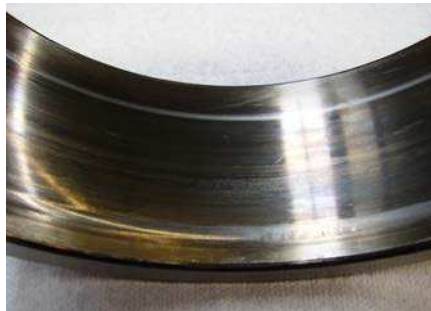
Fig. 1: Path pattern on an outer ring raceway
