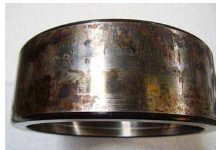
Fig. 4: Fretting corrosion on an outer ring
