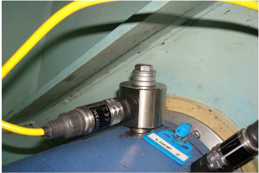
Fig. 11: Radial sensor placement
