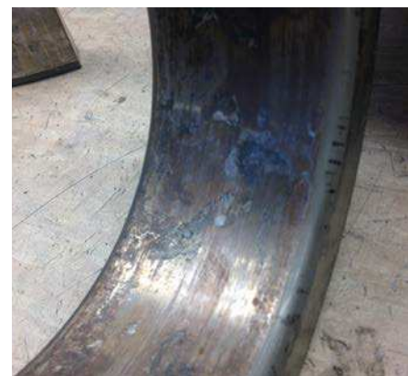
Fig. 8: Evidence of ring creep on a bearing inner ring
