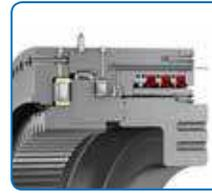
Designed to keep earth out of the main bearing and lubricants in it, SKF main bearing seals are part of a fully integrated large slewing bearing solution. Custom engineered from G-ECOPUR material – a hydrolysis-resistant, self-lubricating proprietary material – these seals are available in many designs, including multi-lip configurations. SKF seals also provide high pressure resistance (up to 10 bar) and can help compensate for misalignments.
