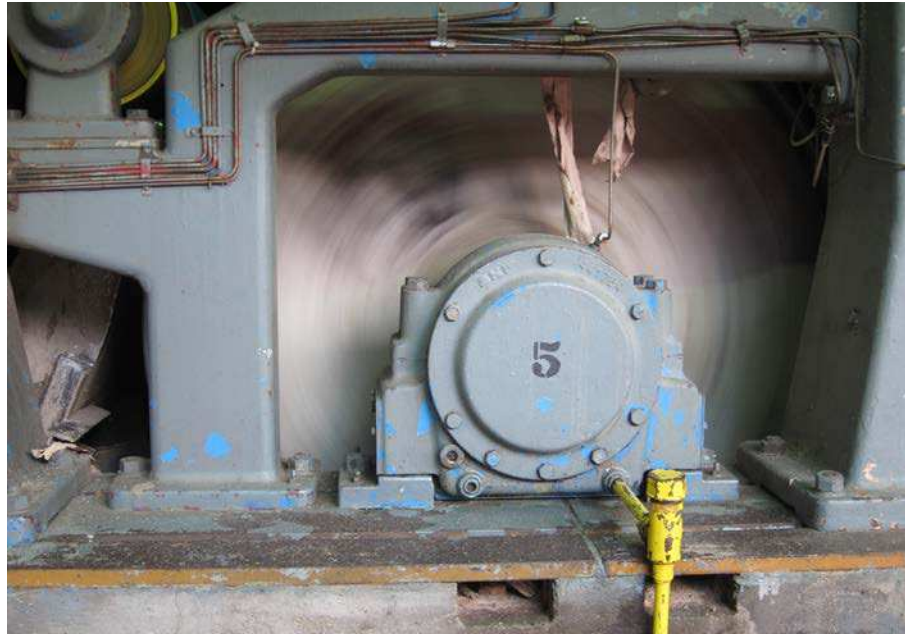
Fig 6: old (48 years old) special SKF 441784, rocker housing supporting drying cylinder bearing. SKF still has the design drawings, but no longer has the casting pattern.
