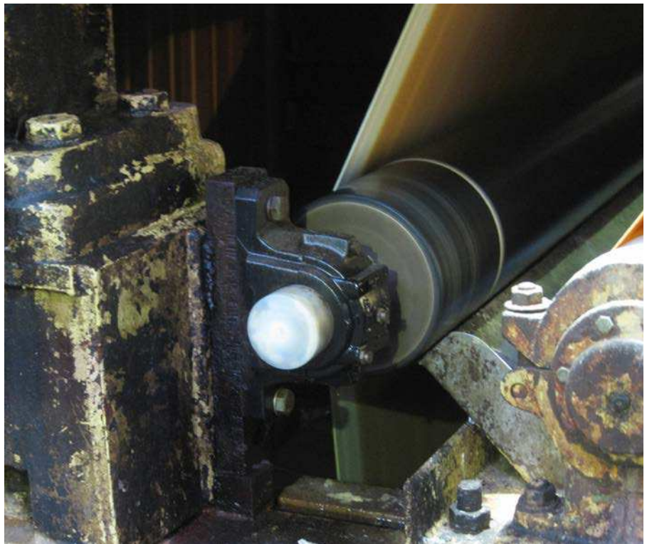
Fig 4: SKF SNL housing used as fabric roll bearing housing.
