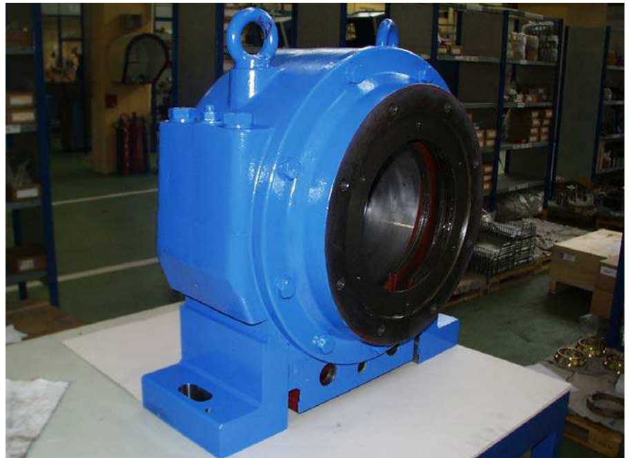
Fig 11: housing of fig 10 rebuild for CARB bearing
