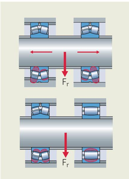
Fig. 8: A traditional plain press roll bearing arrangement with two spherical roller bearings will generate internal axial loads because of the friction and housing deformations. This phenomenon can be eliminated by using CARB as the non-locating bearing.
