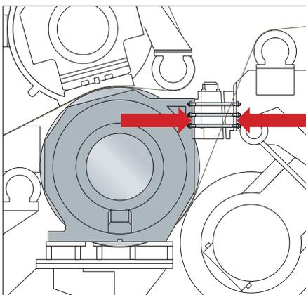
**Fig. 14:** Bearing housing as part of the machine frame. Intermediate piece tightened with large bolts (and high preload force).
