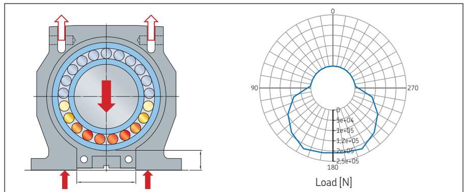
**Fig. 6:** Optimized bearing housing design (optimized gap width, housing thickness and key size).
