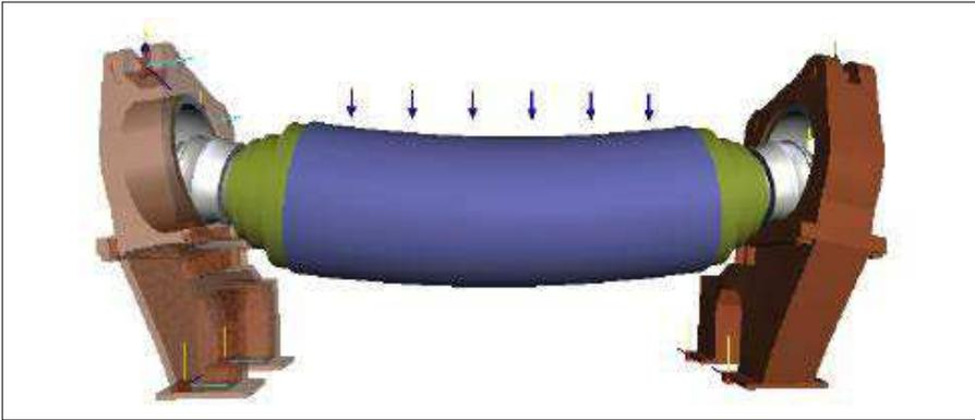
Fig. 7: Advanced bearing calculations made for a high loaded plain press roll with two spherical roller bearings. Internal axial loads are causing the frames to bend.
