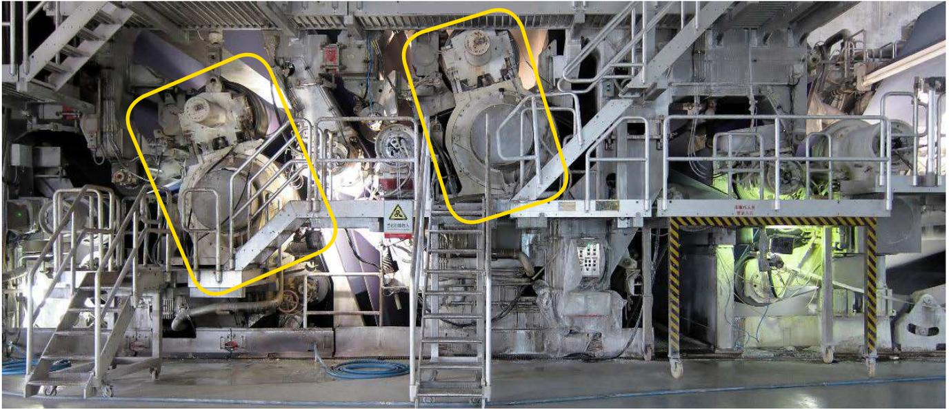
**Fig. 4:** Press section shoe nip, where bearing loads are going through the bearing housing to the counter roll.
