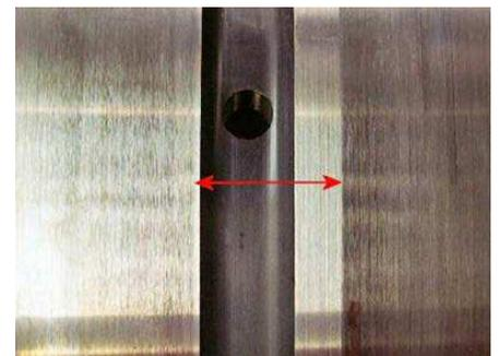
**Fig. 13:** Spherical roller bearing's outer ring's external surface for non-locating (axially free) bearing. The oil lubrication groove position is sharply marked, which shows that the bearing ring has not been moving axially in the housing bore as it should have been.
