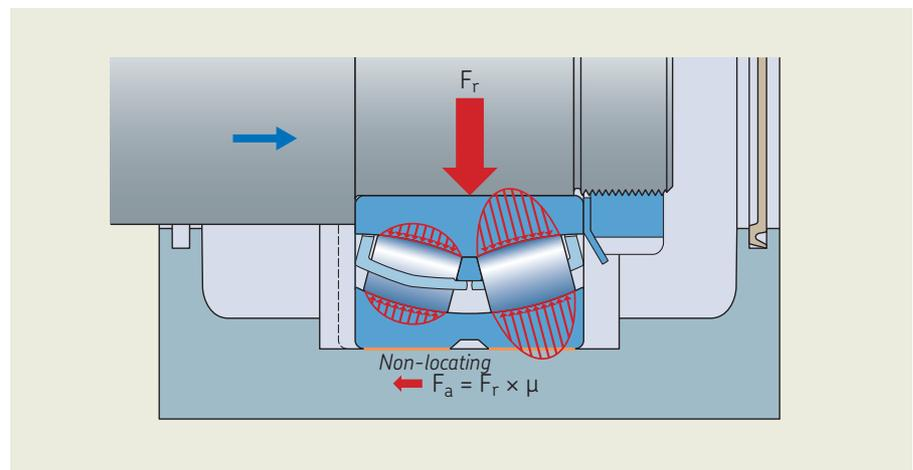
Fig. 10: Axial load generation to spherical roller bearing in an axially free bearing.
