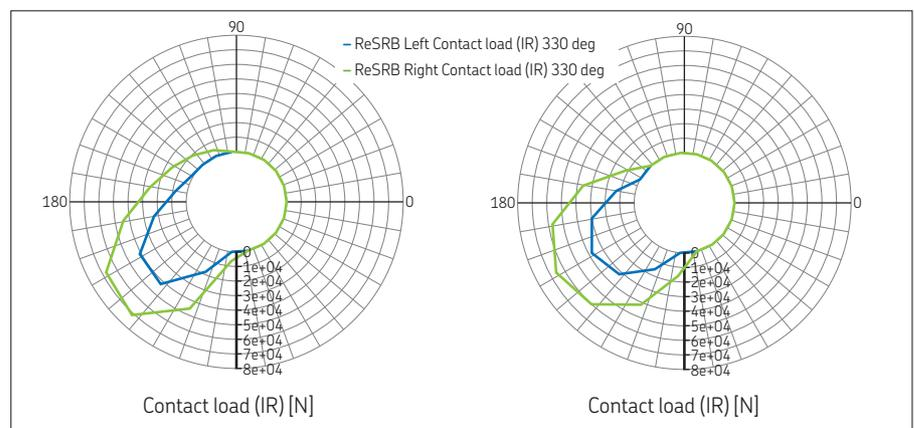
**Fig. 3:** Bearing roller load distribution is wider and maximum load is higher with flexible housing (left) than when calculated with rigid parts (right). SKF Advanced life is 126,000 h with flexible housing, whilst SKF Advanced life with rigid housing is 166,000 h.
