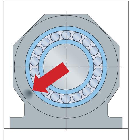
**Fig. 2:** In many cases, the bearing load is exerted on the housing base, but in some cases the bearing load is exerted in a direction where the housing stiffness is changing rapidly.
