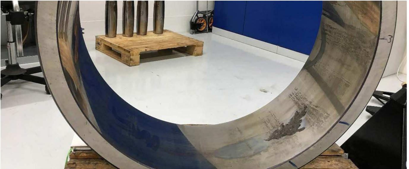
*Fig. 1: Spalling on CARB bearing outer ring raceway due to subsurface fatigue, caused by high load. Standstill corrosion marks generated on raceway during the transportation to failure analysis because of poor corrosion protection.*
