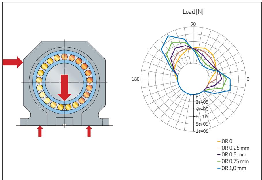
**Fig. 16:** Bearing roller load distribution with different loads caused by an intermediate piece that is too large. SKF Advanced fatigue life with 0 displacement 330,000 h; 0.5 mm 111,000 h; 1 mm 46,000 h.
