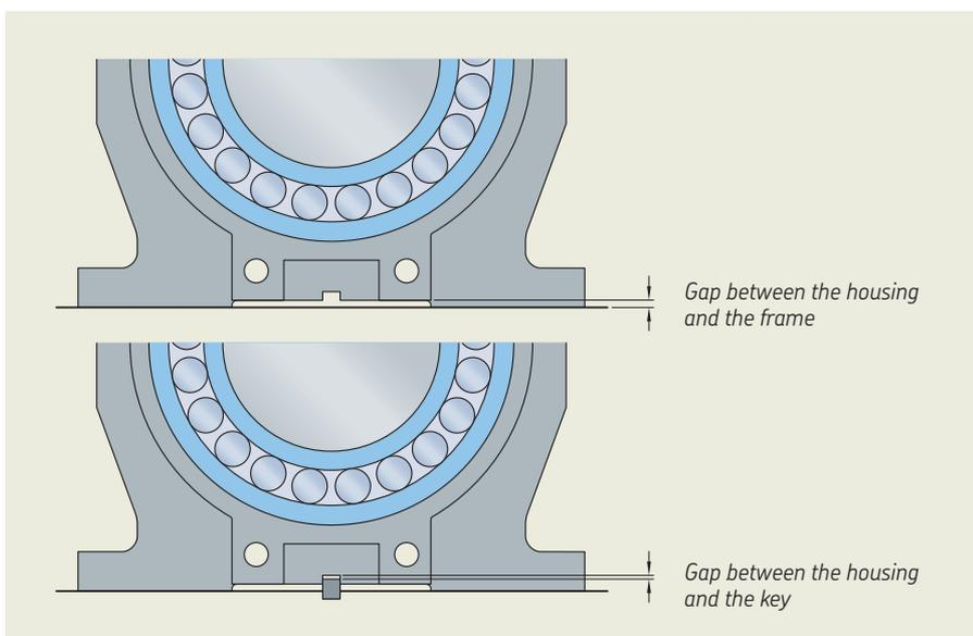
**Fig. 17:** Bearing housing deflection optimized by the use of a gap between the housing and the frame. The gap beneath the housing must also be maintained during use. There must also be a gap between the housing and the key.
