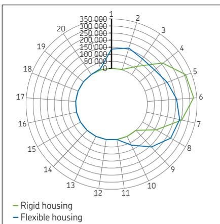
**Fig. 12:** Sample roller load and load distribution with rigid and flexible calculations.
