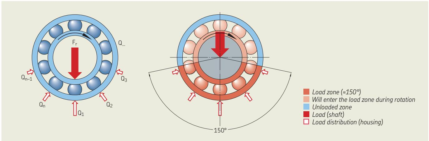
**Fig. 11:** When the bearing is loaded with external load  $F_r$ , bearing load  $F_r$  will be transferred from the inner ring to the outer ring via rollers. The external load will be distributed to rollers. Each roller has an individual roller load ( $Q_n$ ), which is perpendicular to the contact surface. Roller load distribution in the bearing shows how the loads are varied between bearing rollers.
