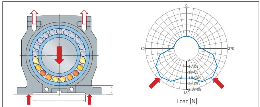
**Fig. 5:** Non-optimized bearing housing design can create two loading zones per bearing.
