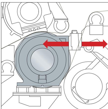
**Fig. 15:** Bearing housing as part of the machine frame. If the thickness of the intermediate piece thickness is too high, it will generate loads that will deform the bearing housing.
