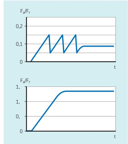
Fig. 9: The upper diagram shows internal axial loads to overcome friction. If axially free bearing movement is prevented by housing deformation, fretting corrosion, dirt, wear particles, etc., the internal axial load can be much bigger than expected (lower diagram).
