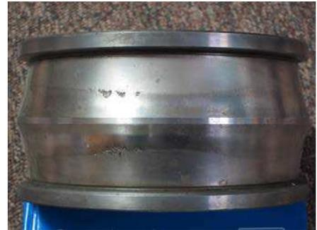
Figure 8: Surface distress and small spalls.
