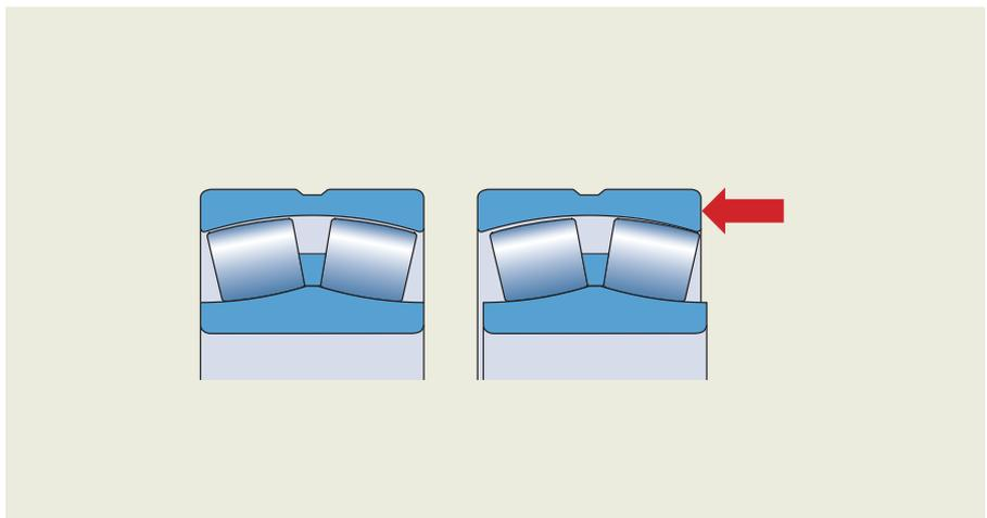
Figure 6: Axially displaced rings affect the radial clearance of each row differently
