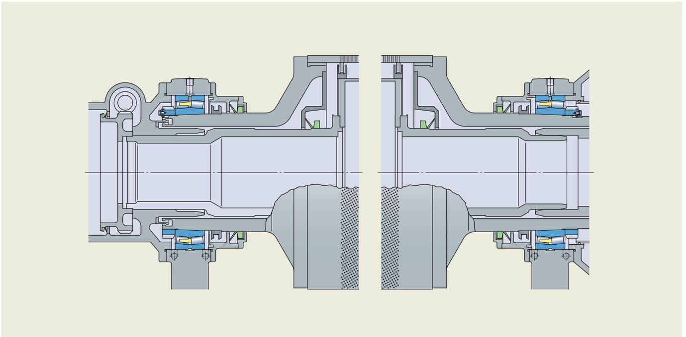
Figure 2: Suction roll with thin-section spherical roller bearings.
