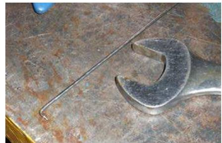
Figure 9: Bent wire with sharp point for feeling surface damages on a bearing.
