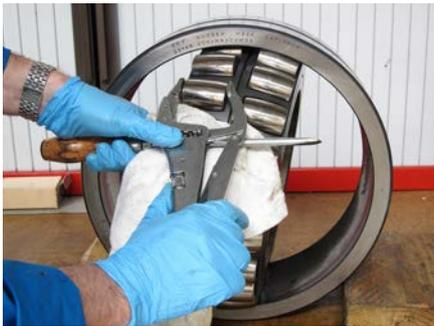
**Fig. 5:** Using the locking pliers as leverage.
