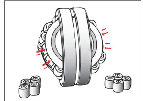
**Fig. 1:** Best practice is to remove four rollers on each side.
