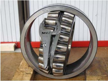
**Fig. 4:** Locking pliers are used to grab one of the rollers.
