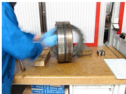
**Fig. 9:** Rolling out the inner ring with rollers and cages.
