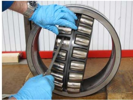
**Fig. 7:** Removing roller with a screwdriver.
