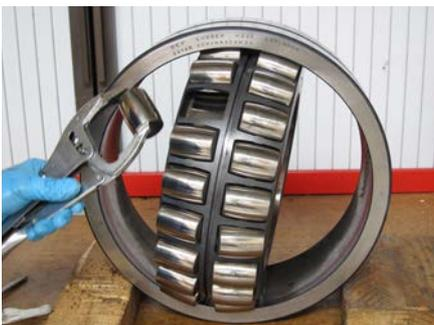
**Fig. 6:** The roller is easily removed.
