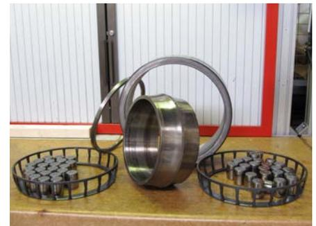
**Fig. 11:** When disassembling, keep rollers from each row together with their half cage.
