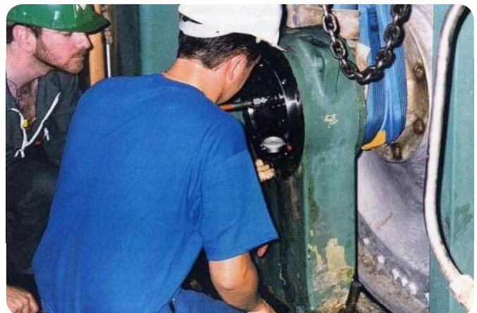
Fig. 2. The first CARB mounted in France. This was at International Paper Saillat using the SKF Drive-up Method. The author is shown on the left.
