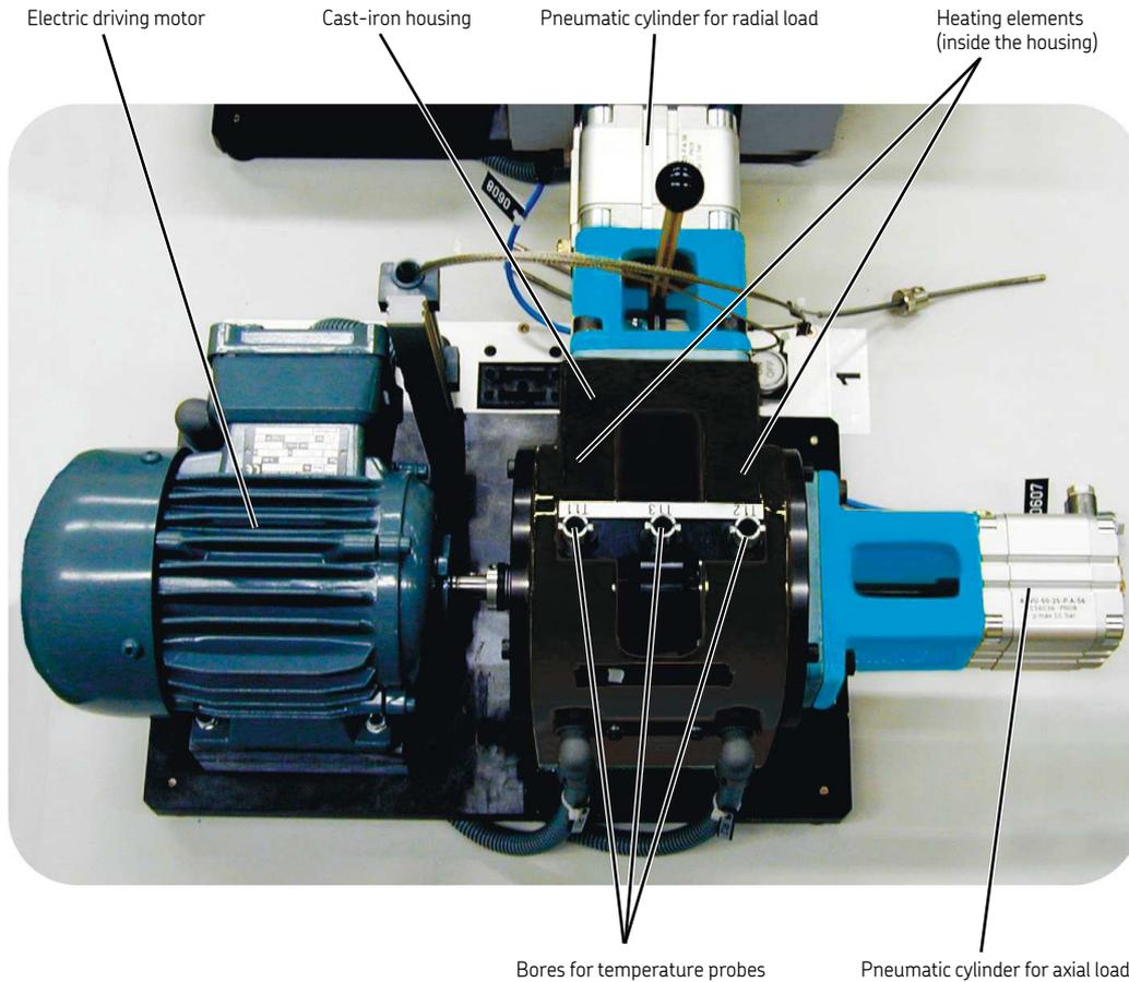
The SKF Grease Test Rig ROF+ essentially consists of two parts – a mechanical test unit and a PC with control and evaluation software. The mechanical unit contains five cast-iron housings. Each housing contains two bearings, mounted on a shaft, the total number of test bearings being ten.
