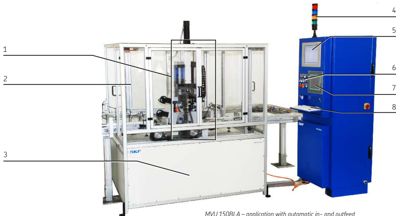
MVU 150BLA – application with automatic in- and outfeed
