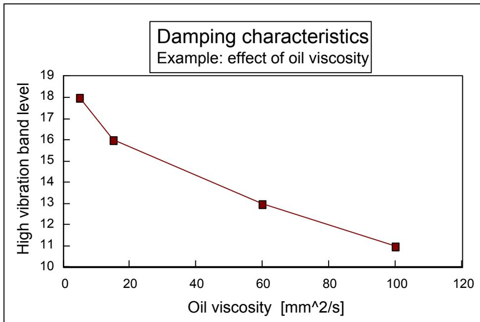
Figure 5: Effect of oil viscosity on damping characteristics
