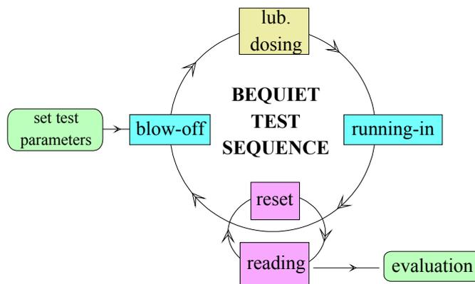
Figure 6: Sequence of BeQuiet + Testing
